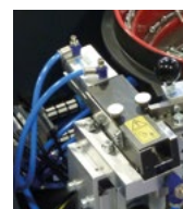
Escapement sensors Control/Secure escapement mechanism
