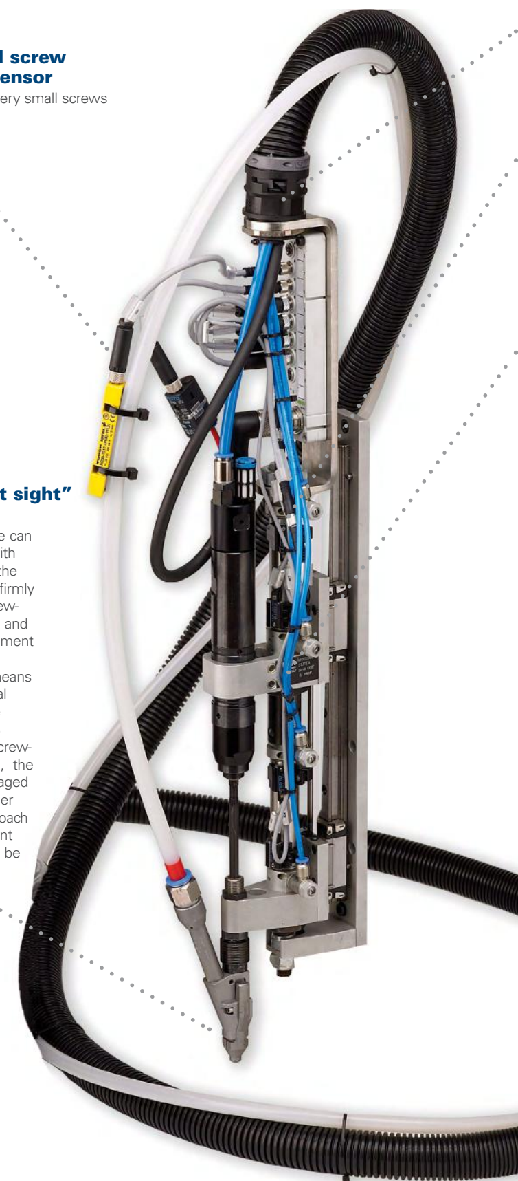
Fastening slide with air nutrunner motor.
