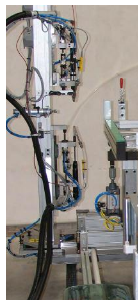
MCA for window frames field: simultaneous top-down and bottom-up assembly
